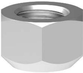
100% crack detected, prevailing torque hexagon nut type according to DIN 980 - V (all-metal design) with a zinc - plated surface. With a plain washer (extra item) suitable for the assembly of lifting points with long threaded bolts for example in through holes.
