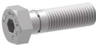
The hexagon socket bolt is with a snap ring so that it can be captively mounted with the ICE-LBG-SR. When used with the ICE-LBG-SR the resulting free thread reach  $H = 12\text{mm}$
