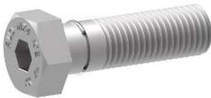
The hexagon socket bolt is with a snap ring so that it can be captively mounted with the ICE-LBG-SR. When used with the ICE-LBG-SR the resulting free thread reach  $H = 18\text{mm}$
