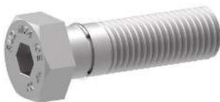
The hexagon socket bolt is with a snap ring so that it can be captively mounted with the ICE-LBG-SR. When used with the ICE-LBG-SR the resulting free thread reach  $H = 24\text{mm}$
