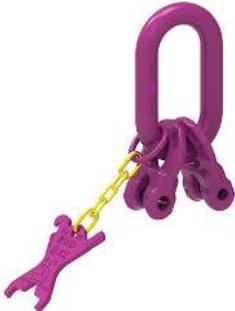
IBK-RG 2 - master link with 2 all direction, movable welded IRG connectors. Thus ensuring that only the correct chain diameter and number of legs can be connected. The ICE load and retaining pins are preassembled. Delivered complete with a flexible, 2-leg identification tag with integrated testing gauge. Surface: ICE-Pink powder coated Manufactured according to DIN EN 1677-4. The internal width is sufficient for high tensile hoist hooks.
