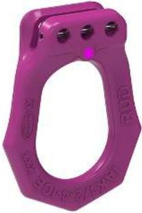
Specially designed , forged master link for the 4mm ICE lifting chain according to DIN EN 1677-4. To be used for a single - leg center connection. Can also be used as an end link (Removal of the ID tag is recommended). Connecting bolt and tensioning sleeve are pre-assembled.
