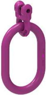
ICE-End link IA-RG 1 with an all direction movable welded IRG connector, thus ensuring that only the correct chain diameter and number of strands can be connected. ISAK-Special master links can be used for this but without ICE-KZA identification tag. The ICE-load and retaining pins are preassembled. Surface: ICE-Pink powder coated ICE-End link is marked by the RUD-ID-TAG<sup>®</sup> (RFID chip) and with the clear identification number distinguished.
