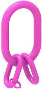
VIP master link without an identification tag and a connector can be used as: VSAK 3/4-20/250 (with VVS-20 and VKZA-20) The size corresponds with that of suspension link type A and B acc. to DIN 5688-3 Manufactured according to DIN EN 1677-4. For crane hooks up to No. 50. DIN 15401.
