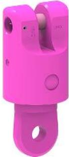
With a ball bearing which enables swiveling under load. Can be versatility combined with all VIP components by means of the clevis connection using the adapter link. Insensitive to dirt owing to the sealed body. Connecting bolt and tensioning sleeve are pre-assembled. The BGR 500/DGUV-Regel 100-500 stipulates that lifting means never be used while in a twisted condition. This requirement is automatically met by the VWA because of the integrated ball bearing.
